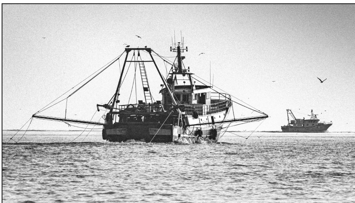
A beam “rapido” trawler in the northern Adriatic Sea; photo by S. Bonizzoni
